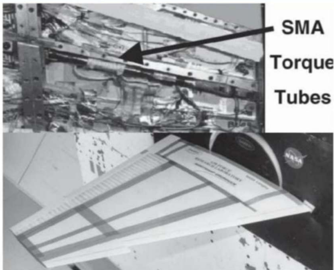
SMA torque tube as installed in the model wing
