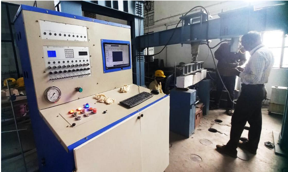
RC beam test in 100 T load frame with Data acquisition
