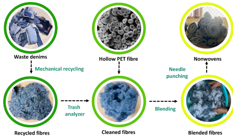
Figure -2: Steps of manufacturing thermal liner using recycled denim fibre
